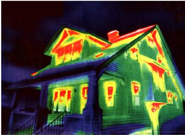
IR image of conductive losses in home
